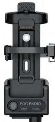
The CK10 Car Kit is a rugged vehicle mounting assembly that enables the PNC380S to be installed on a vehicle dashboard and comply with DOT requirements. The Car Kit allows the PNC380S to be easily removed for handheld job-site communications. The Car Kit includes a locking bracket, an on/off power button, and ports for external speakers, microphones, and push-to-talk buttons. The CARKIT also functions as a docking charger for the PNC380S.
